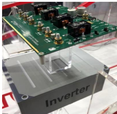
DC-AC Inverter Tr.
